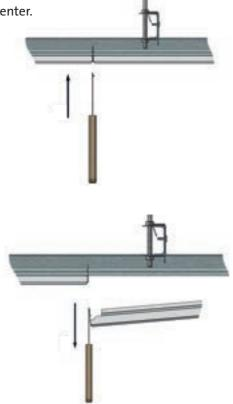
► To unclip the corner of the tile, pull downwards.
