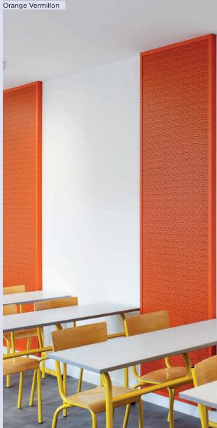
SURFACE AREA: 90 m<sup>2</sup> (41 wall panels standard size 790 x 2700 mm)
