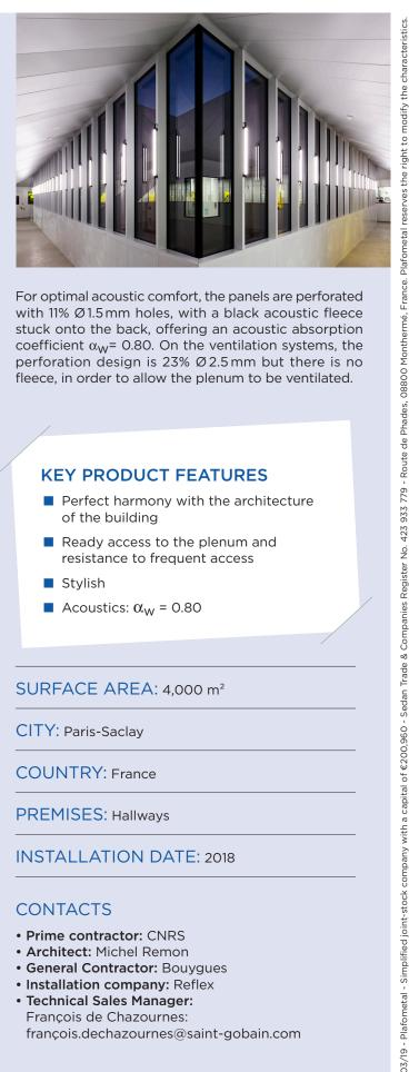
For optimal acoustic comfort, the panels are perforated with 11% Ø1.5 mm holes, with a black acoustic fleece stuck onto the back, offering an acoustic absorption coefficient  $\alpha_W$ = 0.80. On the ventilation systems, the perforation design is 23% Ø 2.5 mm but there is no fleece, in order to allow the plenum to be ventilated.
